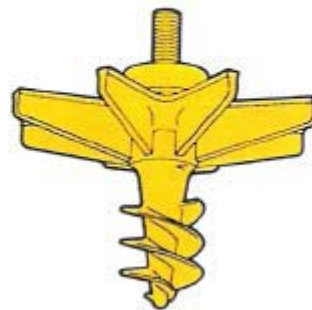
Fig. 4 The combination of tailor-made inducers and impellers, The combination of impeller and inducer with optimization design can reduce NPSHr value.
